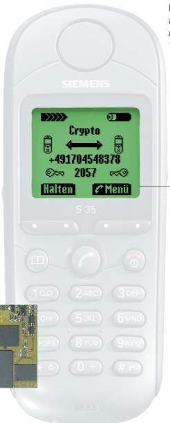
In the crypto mode, your TopSec GSM phone and the called TopSec station automatically agree on a new 128-bit key for each call. The 128-bit key is randomly determined out of  $10^{38}$  possibilities and erased after the call is terminated.
